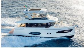
Navetta 52 – the Absolute Appeal – was designed to ensure high levels of cruising comfort in all conditions. The side decks are protected above by a cantilevered superstructure and at the side by sturdy bulwarks. The cockpit terrace is also entirely covered by the flybridge so that it can be enjoyed in any weather. The flybridge is exceptionally large, with a dinette, an outdoor galley, and an aft terrace area with moveable seating for maximum flexibility.
